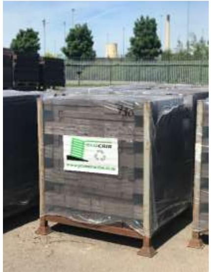
Developed from timber crib technology, the 50mm x 125mm Ecocrib profiles are considerably more durable than treated timber but possess many of the environmental benefits. Ecocrib profiles are manufactured entirely from recycled UK plastic waste with any wastage or surplus material re-processed to form new Ecocrib profiles. Ecocrib can be recycled when it reaches the end of its useful life.
